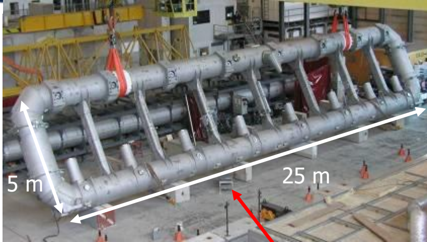
Barrel Toroid (8 coils, 4 T peak, 1080 MJ)
