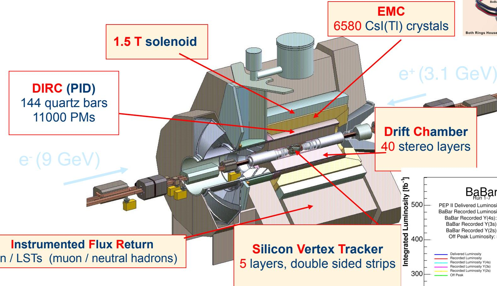
SVT: 97% efficiency, 15  $\mu\text{m}$  z hit resolution (inner layers, perp. track)
