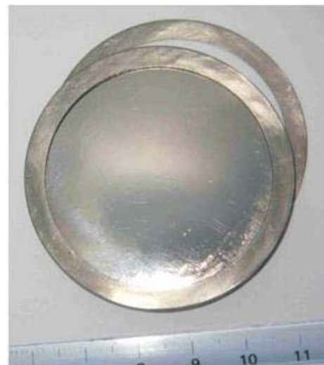
Target from intermetallic compound TiSb
