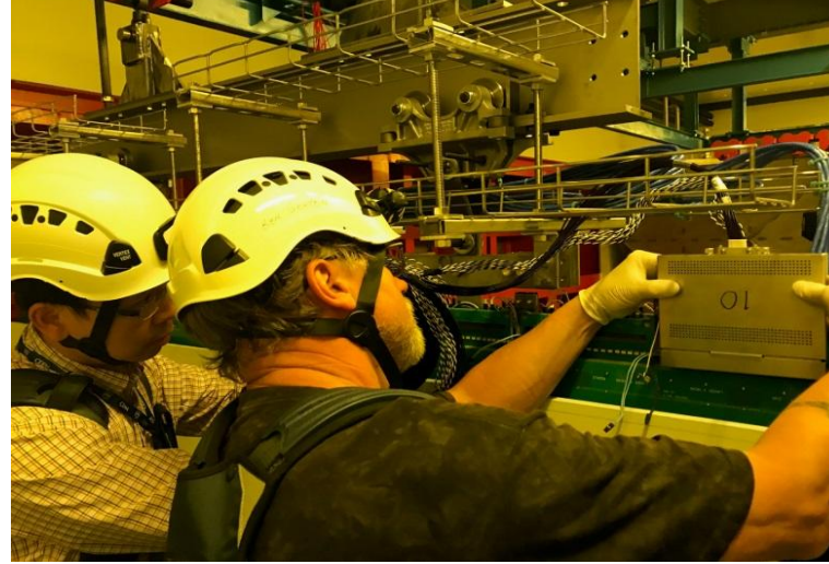
Install CE boxes on the top of APA
