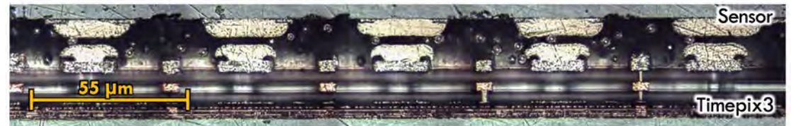
Timepix3-ACF-sensor assembly cross-section
