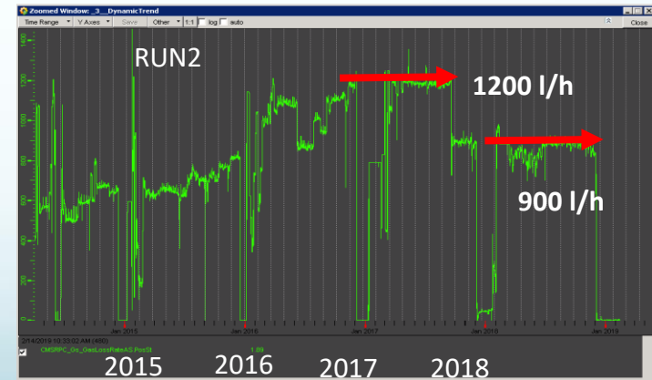
Gas leak monitoring in RUN1 and RUN2
