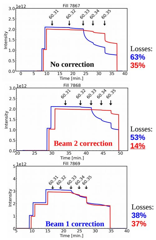
Purpose of this part of MD was to demonstrate the control of the 3Qy resonance and test it with nominal individual bunches before trying high-intensity trains.
