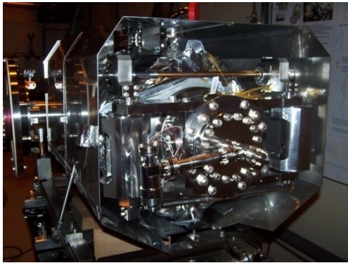
Fully equipped cavity (magnetic shield is open)
