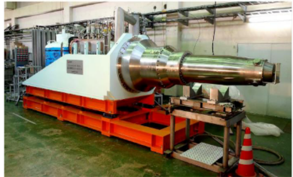
Figure 1: SuperKEKB left side cryostat at KEK.
