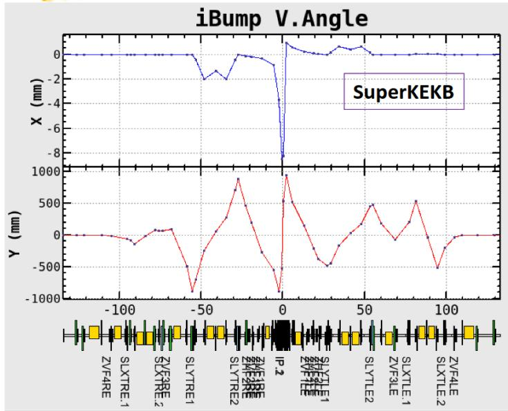
For a vertical angle bump, 8 steering magnets are used in order to close the vertical dispersion.
