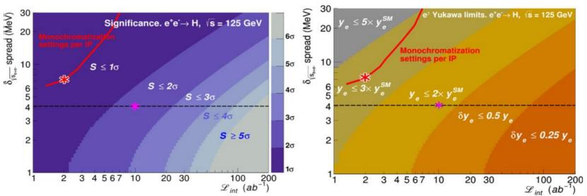
Significance(left) and associated upper limits contours on the electron Yukawa ye. (Right) in the c.m. energy spread vs. integrated luminosity<sup>[1]</sup>
