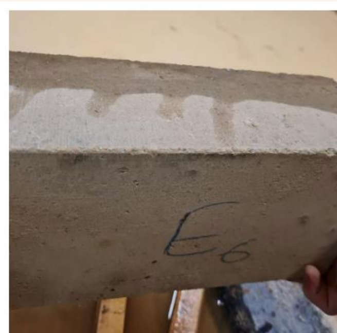
Result of capillarity test
