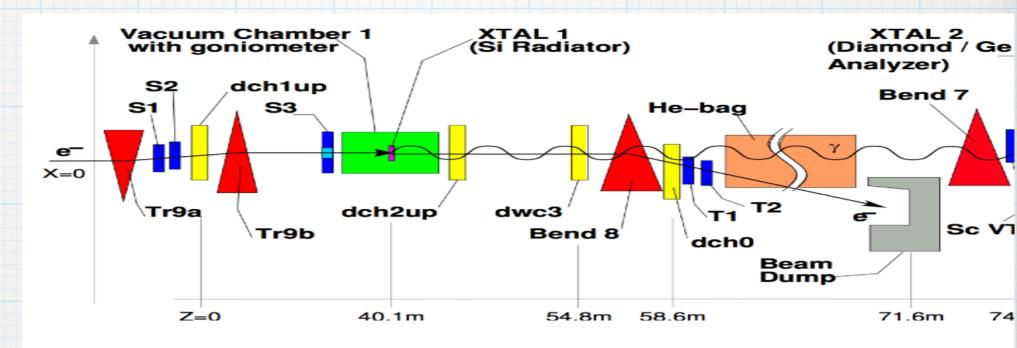
Fig. 1. Setup of the Na59 Experiment
