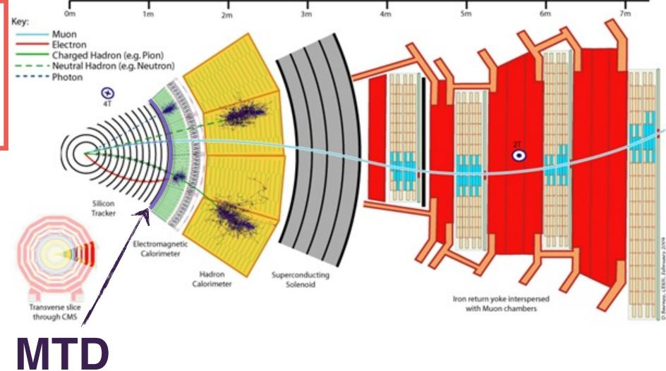
The MIP timing detector (MTD) will have 35 ps resolution at the beginning of its lifetime.
