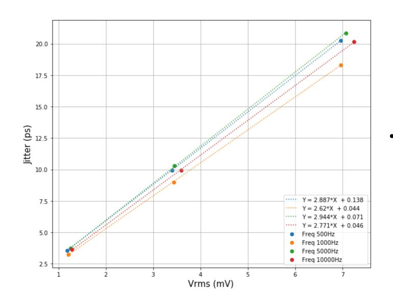
Here the impact of power distribution fluctuations on the timing distribution jitter for an embedded clock distribution chip is quite visible.
