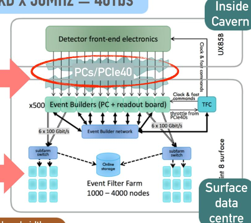
PCIe-gen3: simple protocol, large bandwidth PCIe: maximum flexibility in later networking choice
