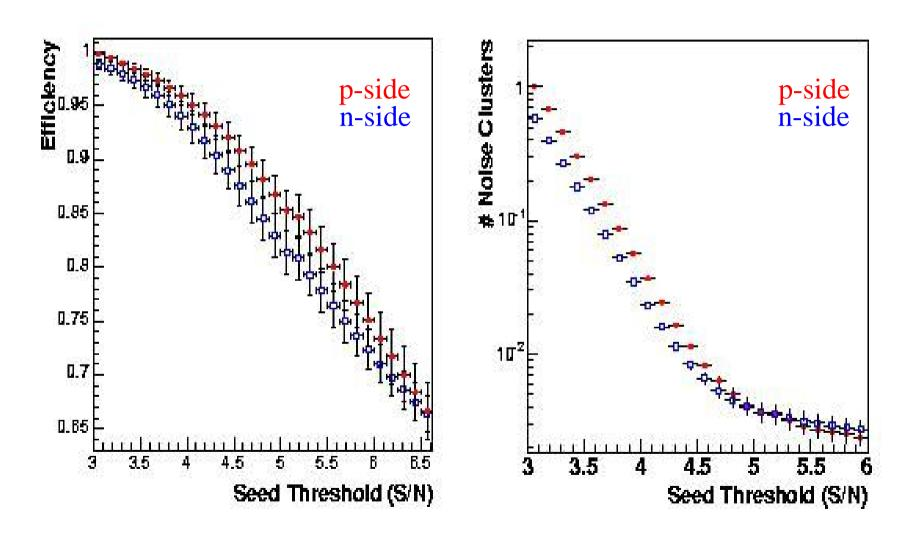
Detection efficiency  $\geq 95\%$  for S/N seed threshold  $\leq 4$
