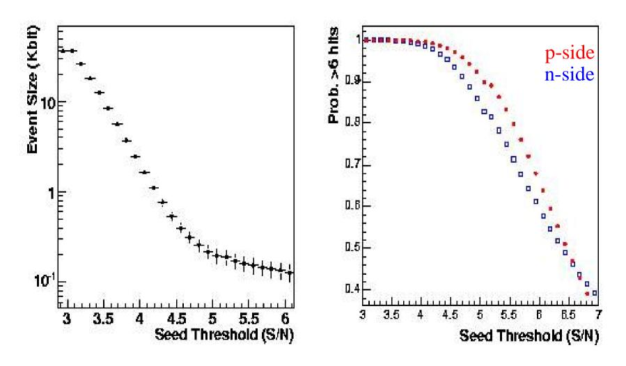
Projected bandwidth 2 Mbit/s, with 1 kHz average trigger rate per orbit  $\Rightarrow$  maximum event size  $\sim$ 2 kbit
