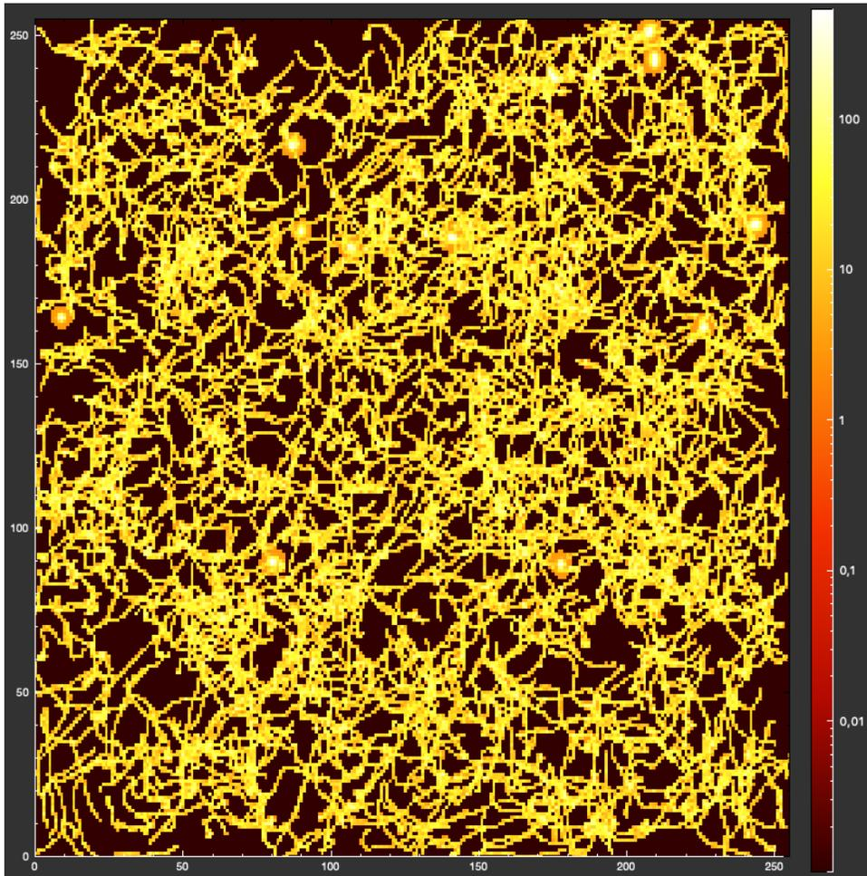
Fast neutrons detected almost exclusively with beam on, practically no fast neutron background.
