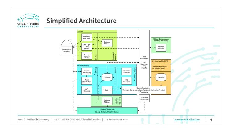
View of the Data Management system with telescope as an input device Far left: near-realtime Prompt Processing Right: High Throughput Computing across multiple sites Bottom and upper right: Dedicated resources for science user access and analysis
