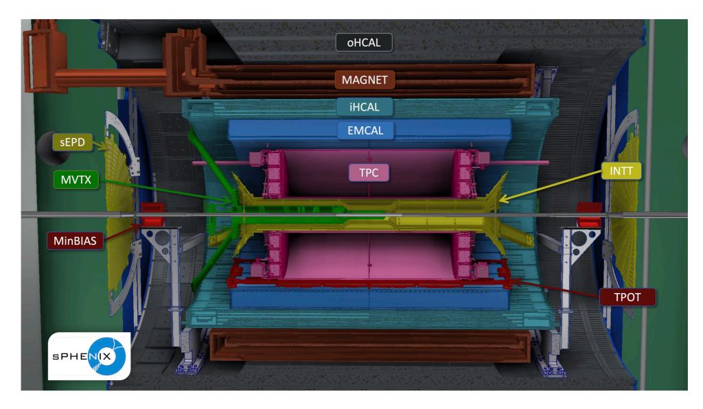
The sPHENIX tracker (1.4 T magnetic field) consists of:
