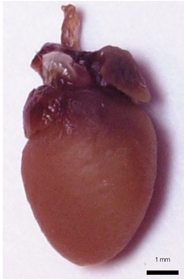
Ethanol-preserved mouse heart scanned using the WidePIX 10x5 detector 60 kVp tungsten spectrum 720 projections, 5 seconds per projection (one hours total) Spatial resolution ca. 7 \mu\text{m} Reconstructed using Voxel, visualized using CTVox and Amide software
