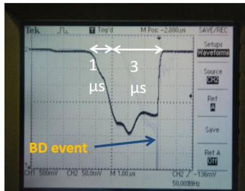
Indirect measurements of field through Faraday Cup
