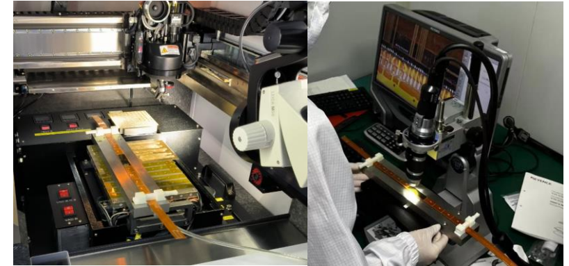
Step 2: Wire bonding - Utilize a vacuumed plate tool to wire bond the TaichuPix-3 chip.
