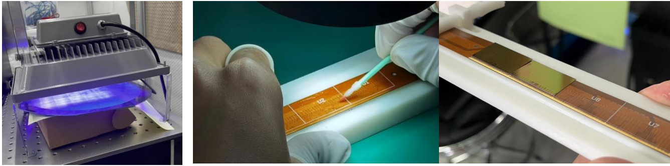
Step 1: Chip fixation - After exposing the chip to UV light, detach it from the blue film and then adhere it to the flexible board using glue.
