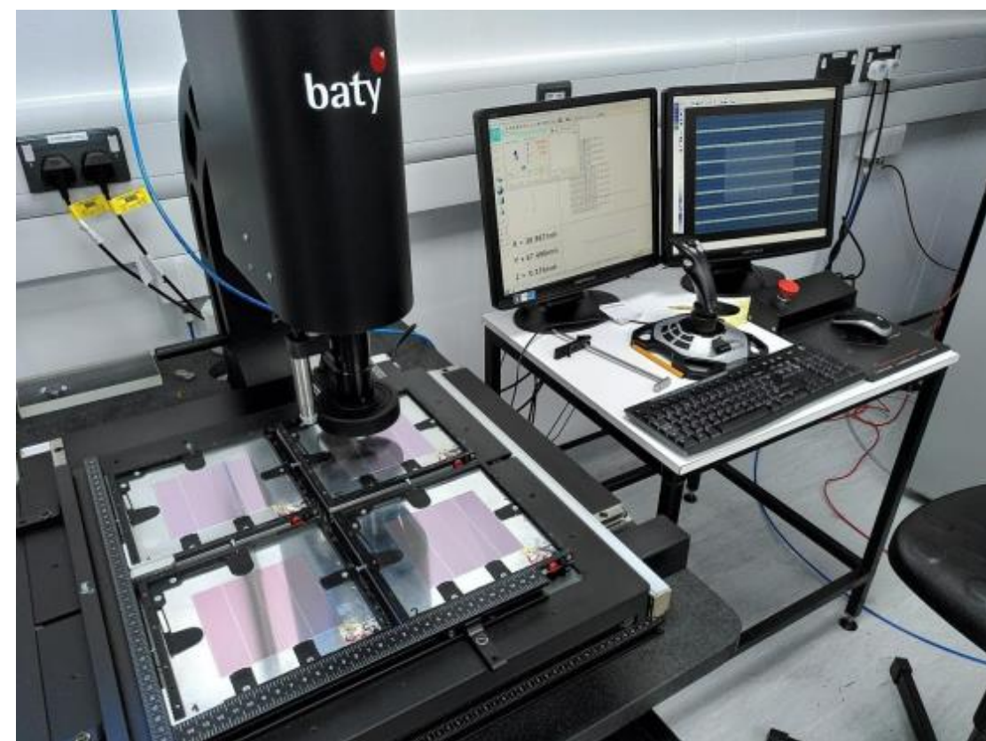
Figure 3. BATY Venture 3030 measurement system installed at University of Cambridge (left) and OGP SmartScope CNC 500 machine used for metrology and Visual Capture tests in Prague (right).
