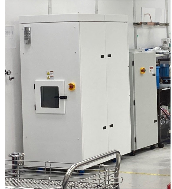
Axom microwave anneal tool in SLAC cleanroom
