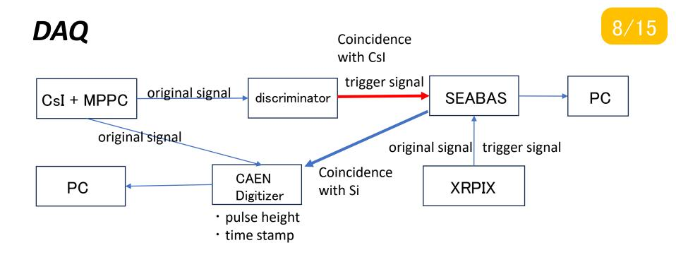
SEABAS is a circuit that receives original signals from XRPIX and trigger signals from MPPC and synchronizes them.
