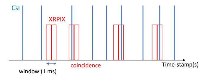
Create a 1 ms window for the XRPIX trigger signal.
