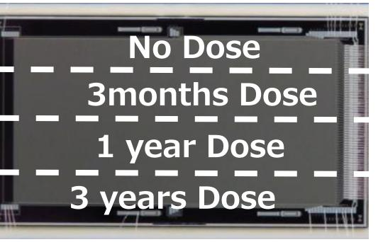
We investigate radiation tolerance of pnCCD by irradiating protons. ✓ 3months, 1 year and 3 years dose at HiZ-GUNDAM orbit.
