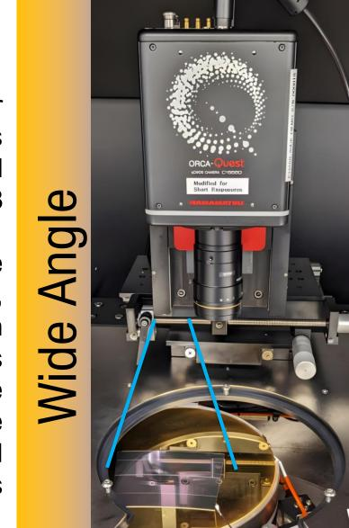
Wide Angle imaging was done with the Kowa LM25XC 25mm lens. This lens provided roughly 0.13x magnification allowing us to image the full surface of the sensor to spot regions of interest while the sensor is breaking down.
