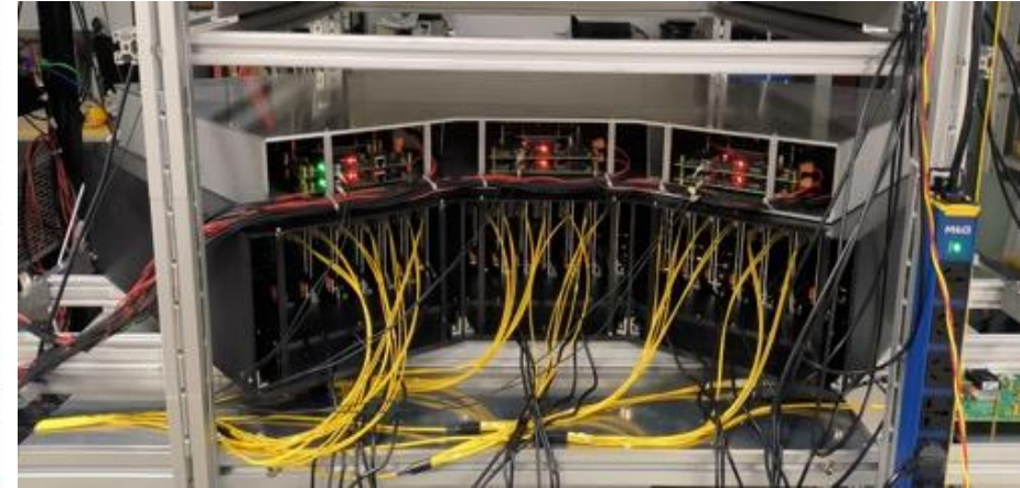
Large-size DIRC detector prototype with full readout
