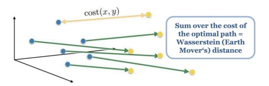
For high statistics a modification can be applied to reduce computation cost: "sliced" EMD
