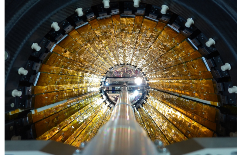
ITS2 Outer Barrel during insertion tests
