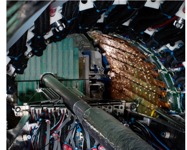
ITS Inner and outer barrels + MFT disk 0 during installation
