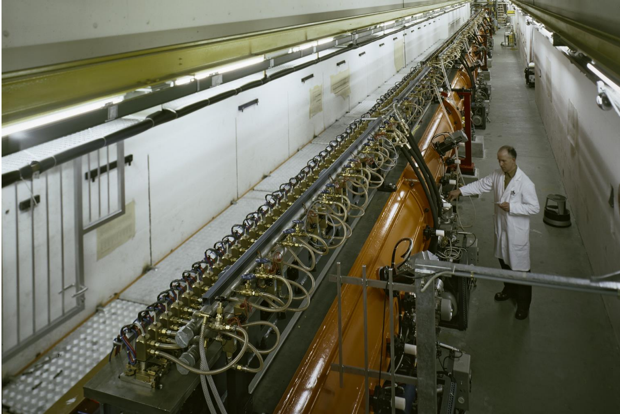
LINAC2 in service from 1978-2018 Accelerating tank 1 shown here provided an energy gain of 10 MeV
