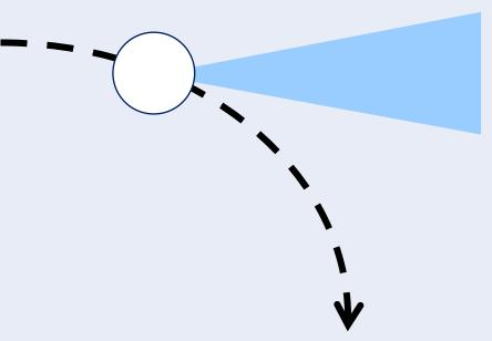
When the trajectory of a charged particle is bent – electromagnetic radiation is emitted, so-called, **synchrotron radiation**
