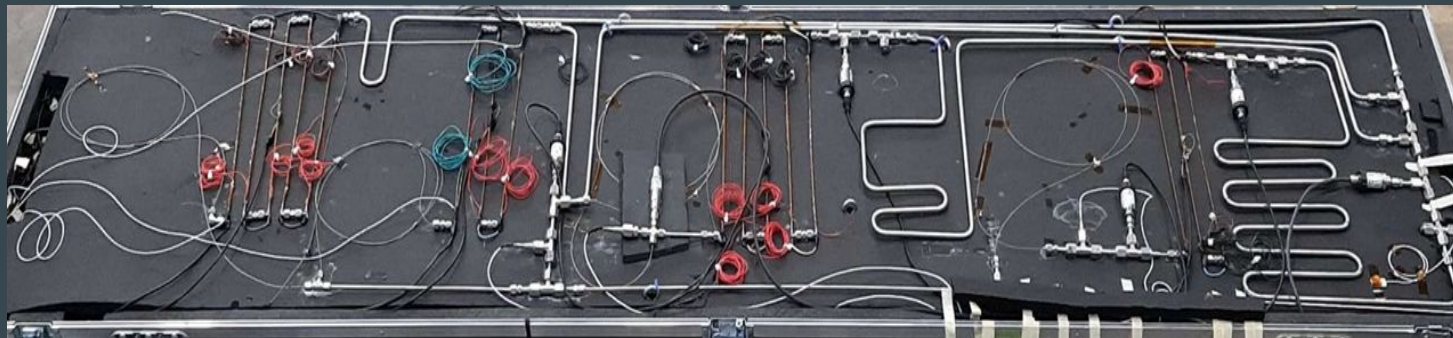
Barrel Cooling Prototype: exact replica of the manifold without flexlines
