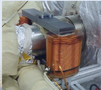
Steel laminated core magnet installed in RHIC
