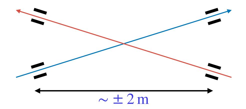
By combining the readings of four BPMs at the both sides of IP for both beams, it is possible to extract the beam-beam deflection.
