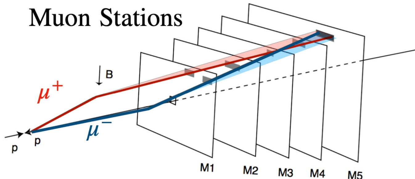
◆ Excellent **MuonID** and  $\mu/h$  already with muon station coincidence
