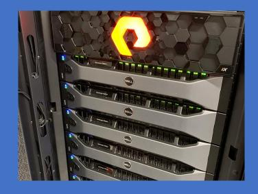
Underpinning DAFNI is a dedicated High Throughput Computing (HTC) Cluster which is comprised of 27 nodes and a total of 792 CPU's, backed by a working memory of 16.8 TB.
