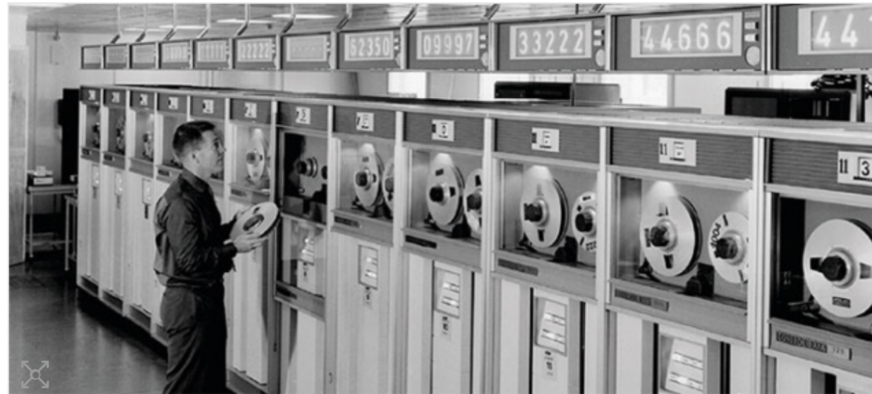
The tape-unit reel-display system (RDS) shown mounted over tape units in the 6600 computing complex, in 1965.
