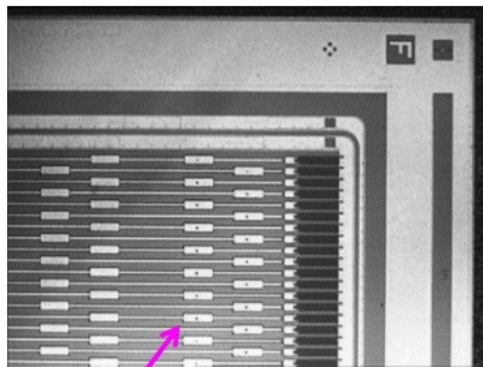
Metalisation above strips, with bond pads
