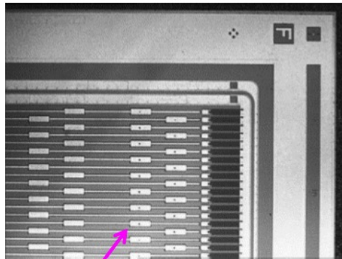
Metalisation above strips, with bond pads
