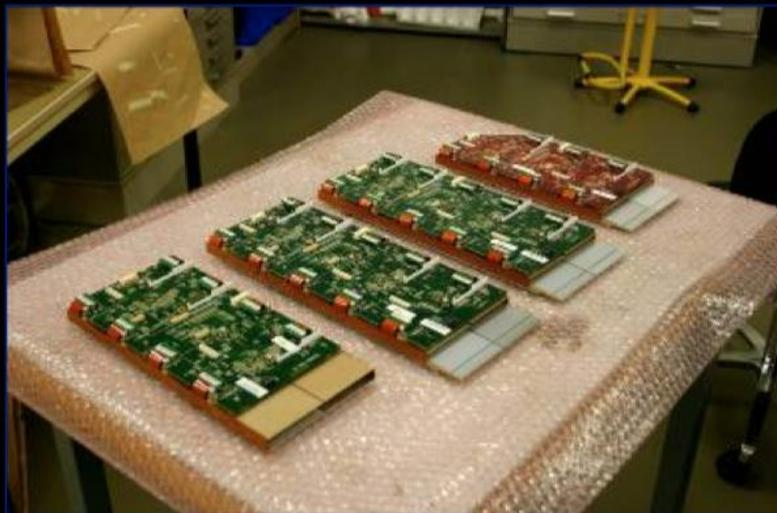
3 types of "ladder" filled with Si sensors
