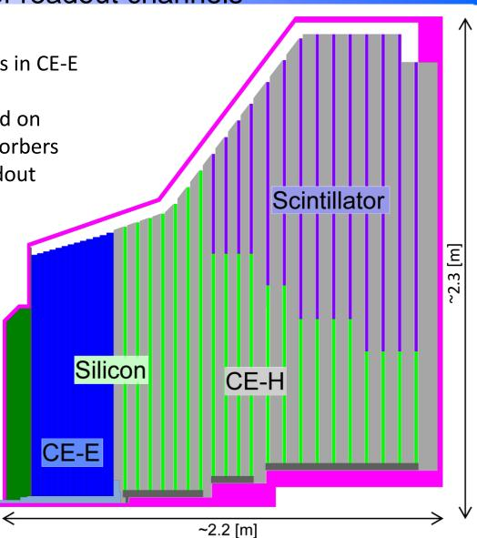
Electromagnetic calorimeter (CE-E): Si, Cu & CuW & Pb absorbers, 26 layers, 25 X<sub>0</sub> & ~1.3 $\lambda$ Hadronic calorimeter (CE-H): Si & scintillator, steel absorbers, 21 layers, ~8.5 $\lambda$  7
