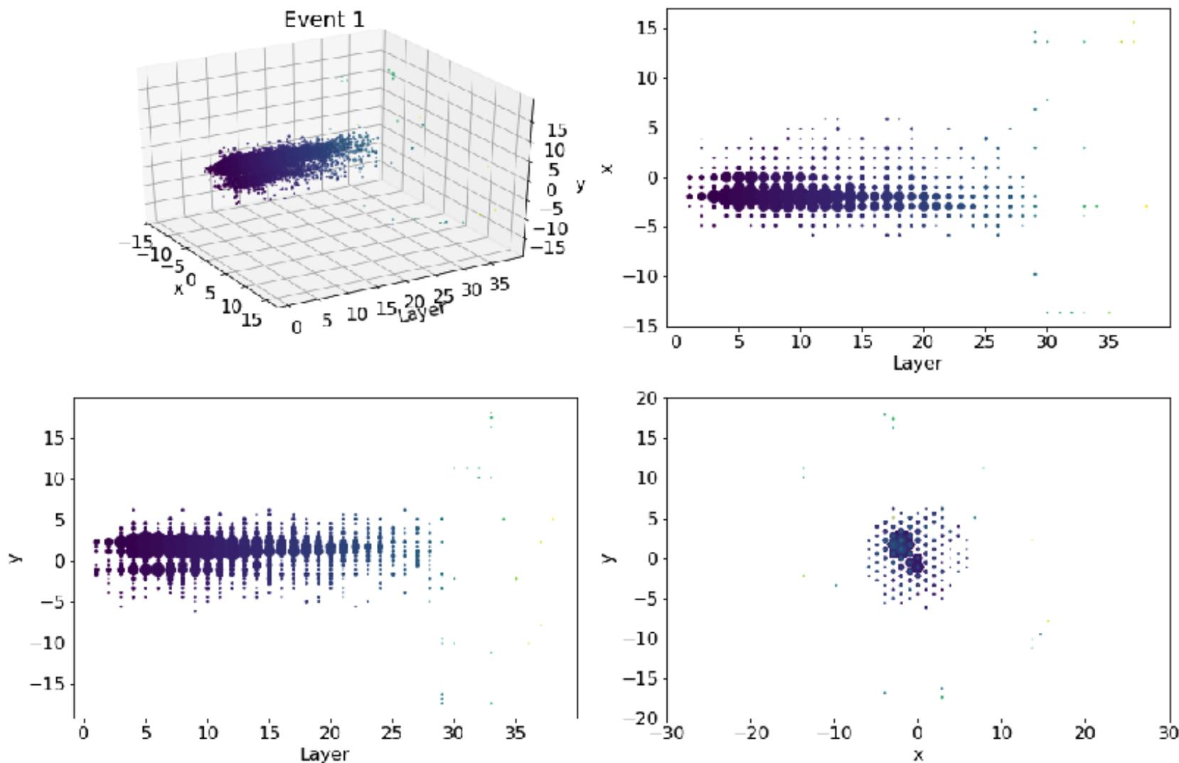
2 energy clusters seen due to **electron bremsstrahlung** upstream of HGCal
