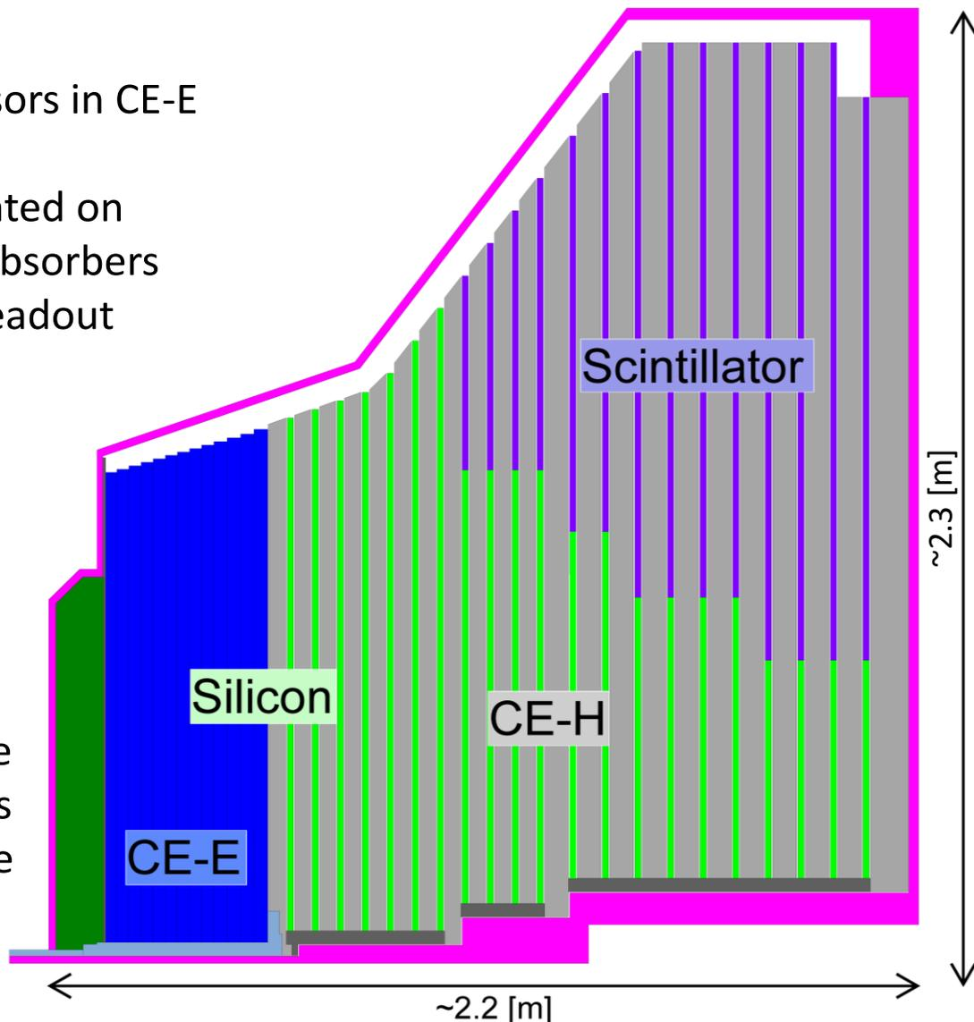
Electromagnetic calorimeter (CE-E): **Si**, Cu & CuW & Pb absorbers, 26 layers,  $25 X_0$  &  $\sim 1.3\lambda$
