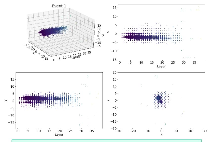
2 energy clusters seen due to **electron bremsstrahlung** upstream of HGCAL
