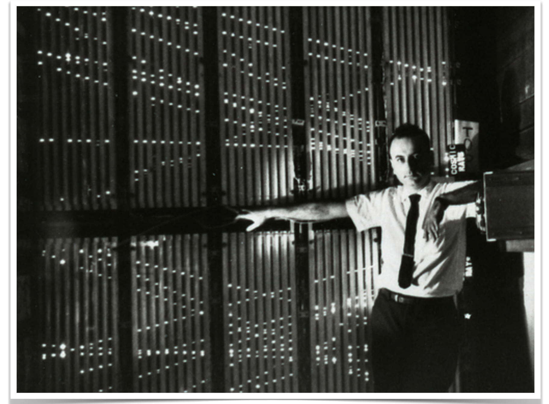
Mark Schwartz showing off the “spark chamber”, where the muon neutrino was directly observed
