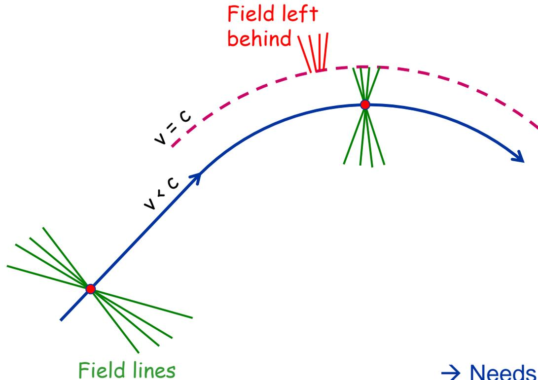
Synchrotron radiation is caused by leaving part of fields behind when the beam moves along the curve.
