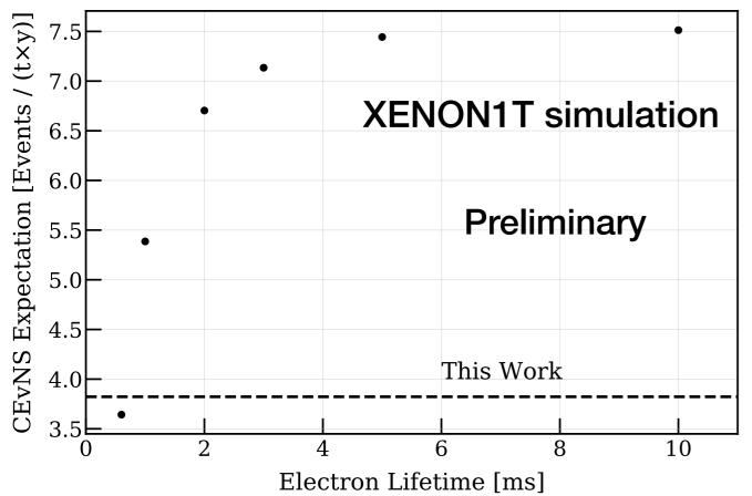
Increasing light and charge detection efficiency is critical (e.g. electron lifetime)
