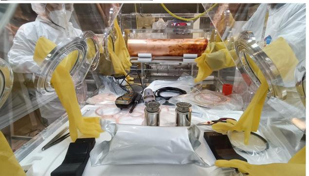
Operation for Nal-37 in underground Radon-free clear room (400mBq/m<sup>3</sup>) previously built for DarkSide-50
