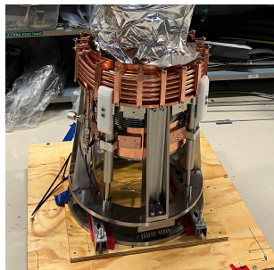
New cooling coil. Relies on conduction to cool critical components.
