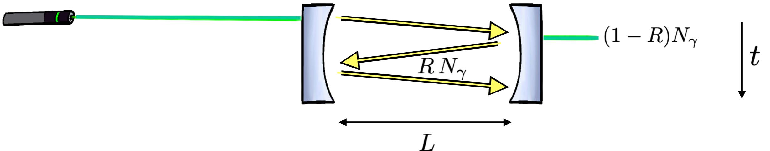
$$\frac{dN_\gamma}{dt} \simeq \frac{\Delta N_\gamma}{L/c} = \frac{c(1-R)}{L} N_\gamma \quad \rightarrow \quad \tau_\gamma^{-1} \equiv \kappa \simeq \frac{c}{(1-R)^{-1} L}$$
