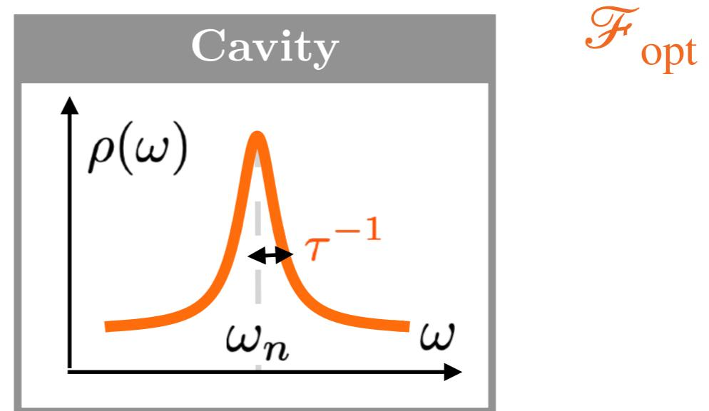
$$\rho(\omega) = \sum_i \delta(\omega - \omega_i) = \sum_n \frac{1}{2\pi} \int dt e^{i(\omega - \omega_n)t} e^{-t/(2\tau)} = \sum_n \frac{\tau^{-1}/2}{(\omega - \omega_n)^2 + (\tau^{-1}/2)^2}$$
