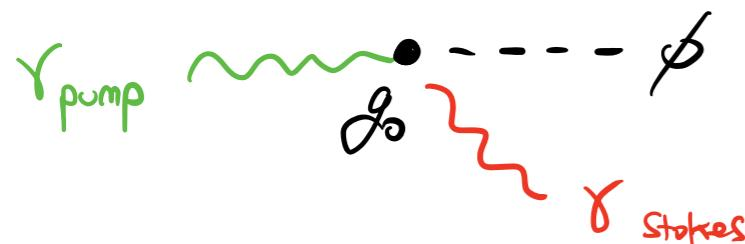
$$\vec{p}_{\gamma 1} = \vec{p}_\phi + \vec{p}_{\gamma 2}$$
