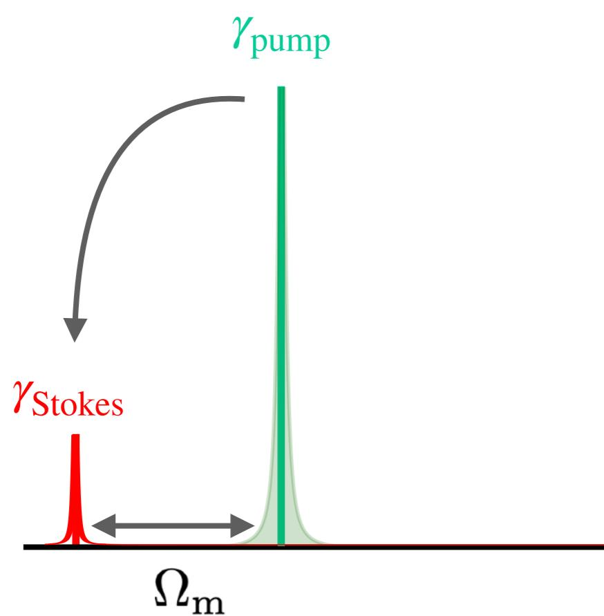
$$\omega_{n_{\text{mec}}} = n \frac{\pi}{L} c_s, \quad n \subset \mathbb{Z}$$
