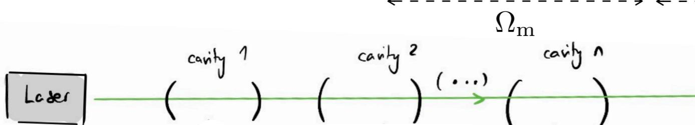
$$\frac{\delta P_{\text{filtered}}}{\delta P_{\text{input}}} = \left( \frac{1}{1 + (\omega/\kappa)^2} \right)^n$$
