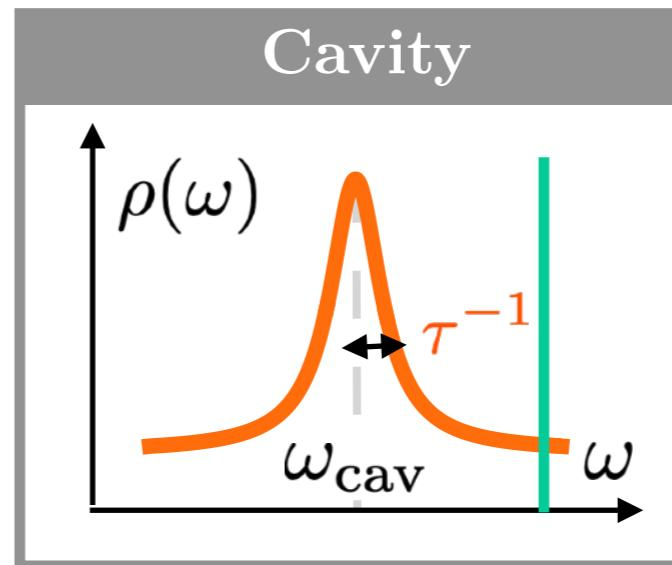
$$\rho(\omega) = \sum_i \delta(\omega - \omega_i) = \sum_n \frac{1}{2\pi} \int dt e^{i(\omega - \omega_n)t} e^{-t/(2\tau)} = \sum_n \frac{\tau^{-1}/2}{(\omega - \omega_n)^2 + (\tau^{-1}/2)^2}$$
