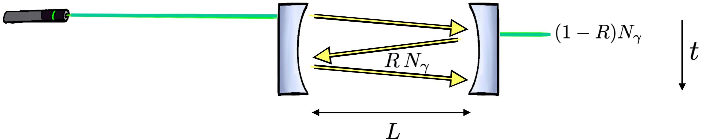
$$\frac{dN_\gamma}{dt} \simeq \frac{\Delta N_\gamma}{L/c} = \frac{c(1-R)}{L} N_\gamma \quad \rightarrow \quad \tau_\gamma^{-1} \equiv \kappa \simeq \frac{c}{(1-R)^{-1}L}$$
