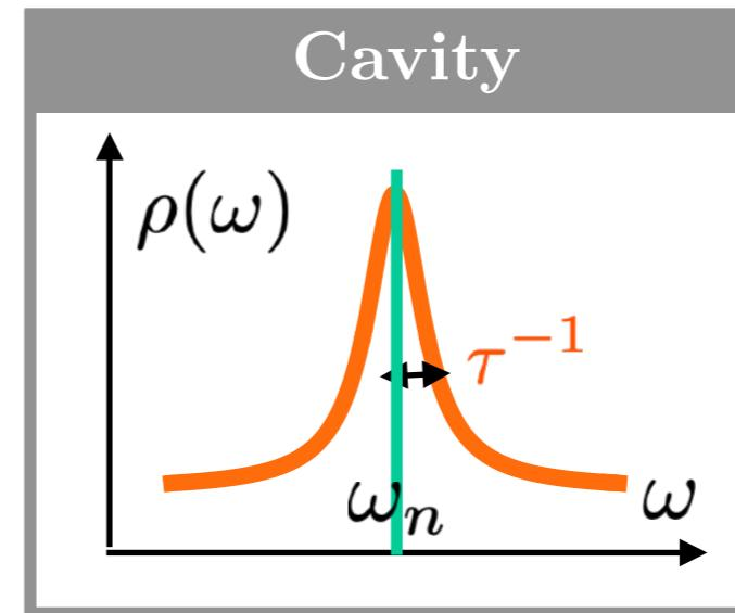
$$\rho(\omega) = \sum_i \delta(\omega - \omega_i) = \sum_n \frac{1}{2\pi} \int dt e^{i(\omega - \omega_n)t} e^{-t/(2\tau)} = \sum_n \frac{\tau^{-1}/2}{(\omega - \omega_n)^2 + (\tau^{-1}/2)^2}$$
