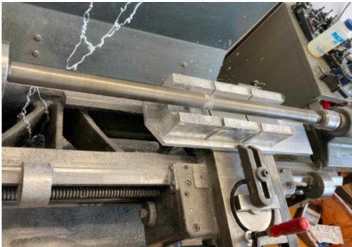
Tooling for first test made on conventional machines
