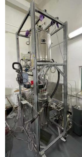
cryogenic and purification system
