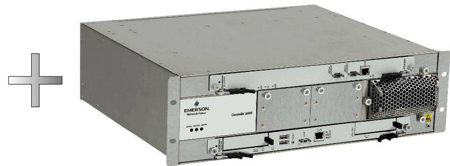
Centellis 2000 from Emerson AdvancedTCA Platform 2 slots + ShManager
