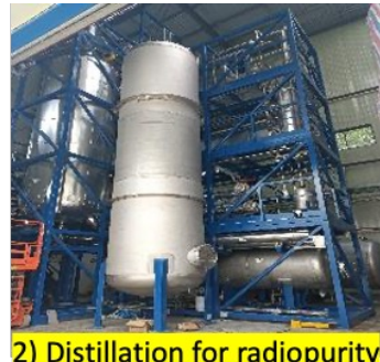
2) Distillation for radiopurity
